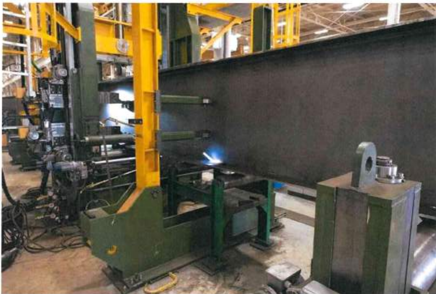
An automated machine makes a continuous weld at the Cimolai-HY facility in North Olean. Bob Clark/Olean Times Herald
